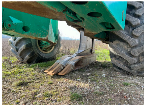
Image, left: using the ploughing method, even long pipe sections can be laid in the shortest possible time and with significantly less environmental impact; image, centre: the ploughshare with the displacer is the so-called leading edge when it comes to underground installation; image, right: to create the extensive piping system, several pipe sections with up to 60 pipes were interconnected using the heated-tool butt welding method
