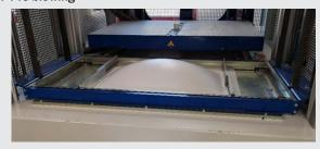
Forming process (here: vacuum forming; other forming methods possible)
